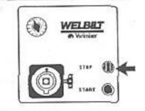
Stop the mixer by pressing the red stop button <STOP>
